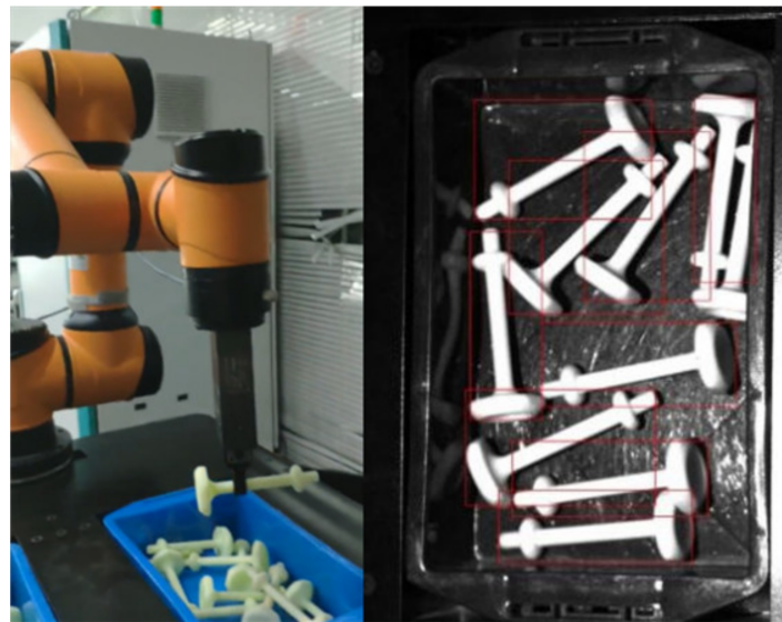
Figure 10. The hand–eye relationship was verified via grasping experiments. It was found that the gripper could accurately grasp the defined position in the target. Although there were occasional deviations, they were still in the operating space of the gripper and could be successfully grasped during the experiment.
