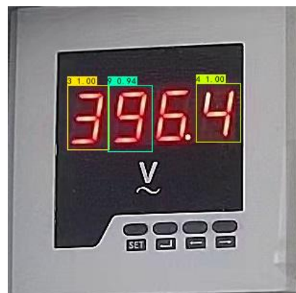
Figure 12. Schematic diagram of missed detection of number "6.".
