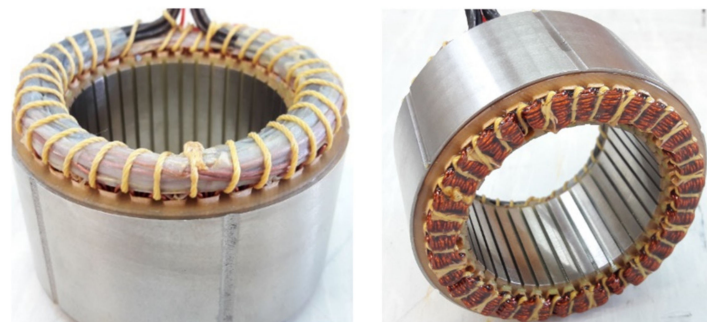
Figure 8. Example of laying the motor cables in individual tubes and assembling them vertically from the winding ends in order to avoid any overlapping.
