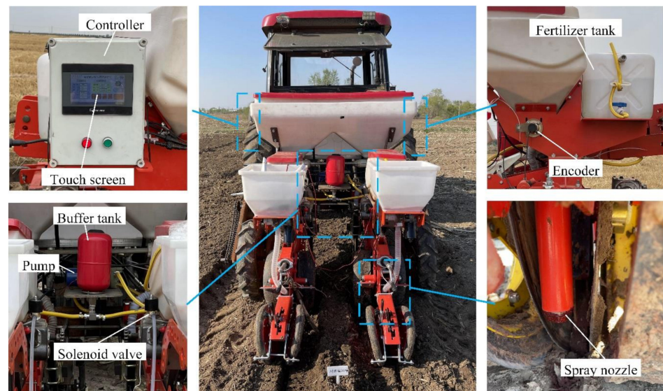
Figure 7. The field experiment with the double-row precise application system for liquid starter fertilizer.
