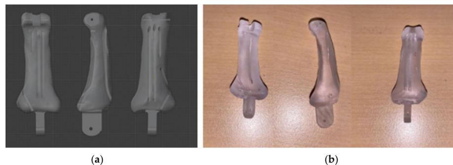
**Figure 4.** Design of tendons and tunneled tube in bone: (a) 3D model; (b) 3D printed bone.
