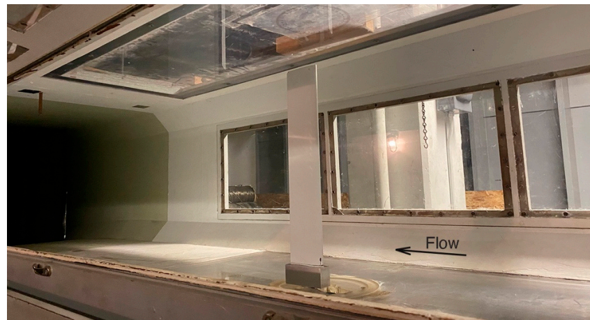
Figure 12. DAP wing mounted in the 21 \times 30'' ( 53.3 \times 76.2 cm) wind tunnel at the University of Kansas (USA) Aerospace Engineering Department.
