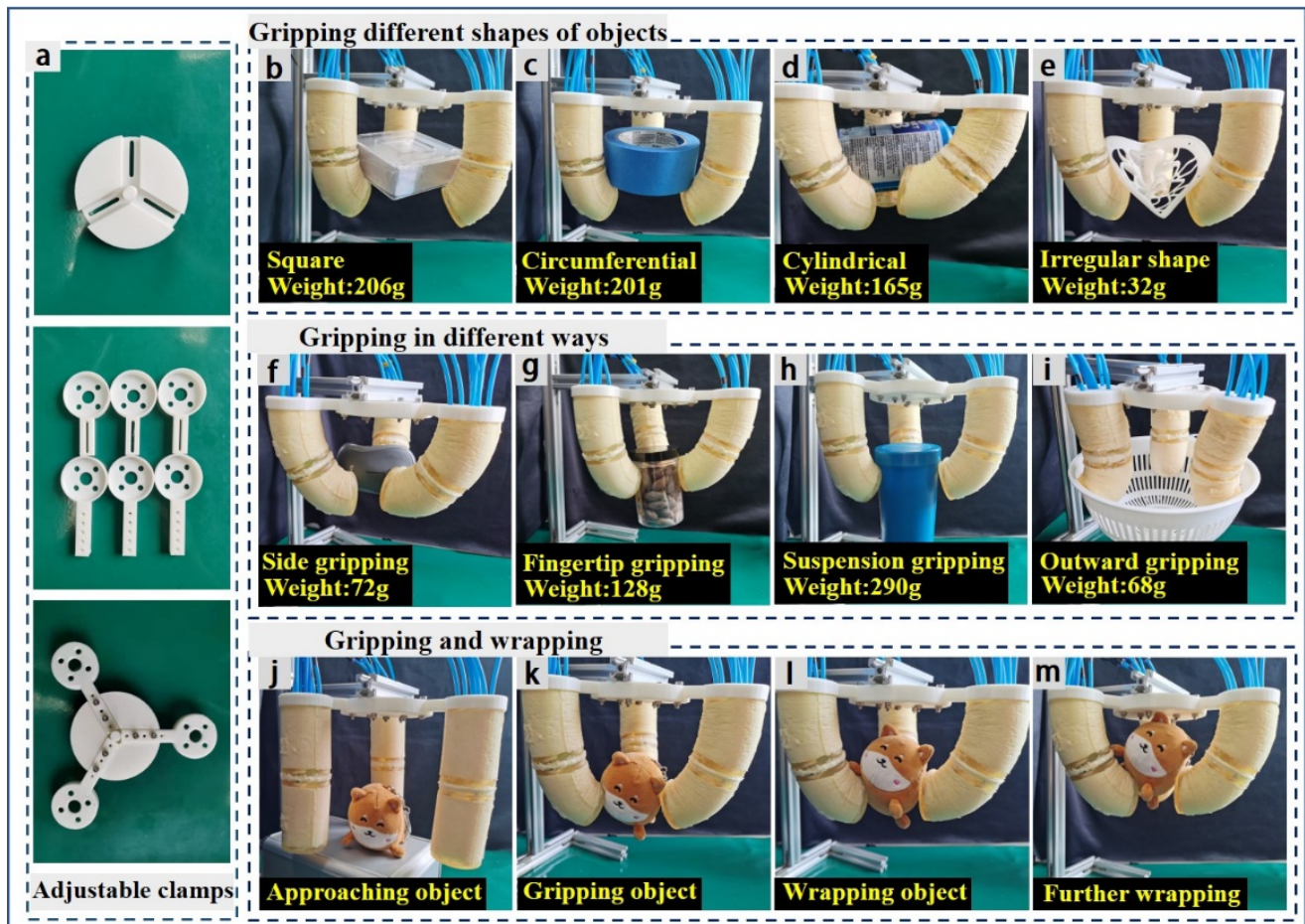
Figure 11. Soft robot used as a soft gripper: (a) adjustable clamps; (b–e) gripping square, circular, cylindrical, and irregularly shaped objects; (f–i) gripping objects by the side, fingertips, suspension, and outward pressure; (j–m) gripping and wrapping plush toys.
