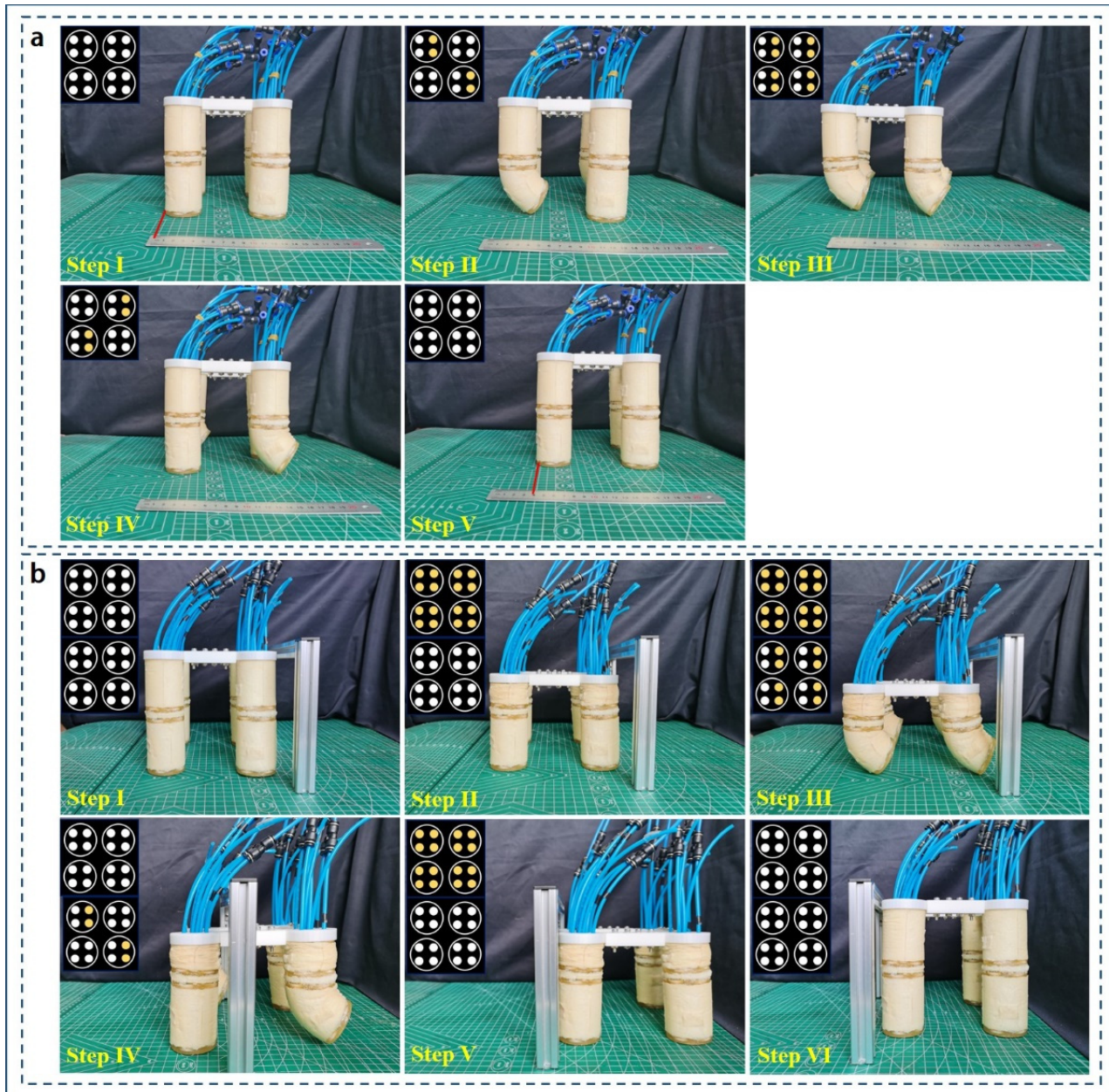
Figure 12. Quadruped-like soft robot: (a) Walking process and the corresponding pumping sequence; (b) obstacle avoidance process and the corresponding pumping sequence (yellow: pumping, white: no air pressure).
