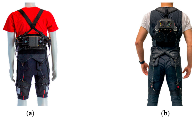
Figure 7. Comparison of the actuation pack of the hip-extension exosuit. (a) Exosuit designed by Harvard University [5]. (b) Renewed Exosuit, based on the proposed PEQDD actuators.
