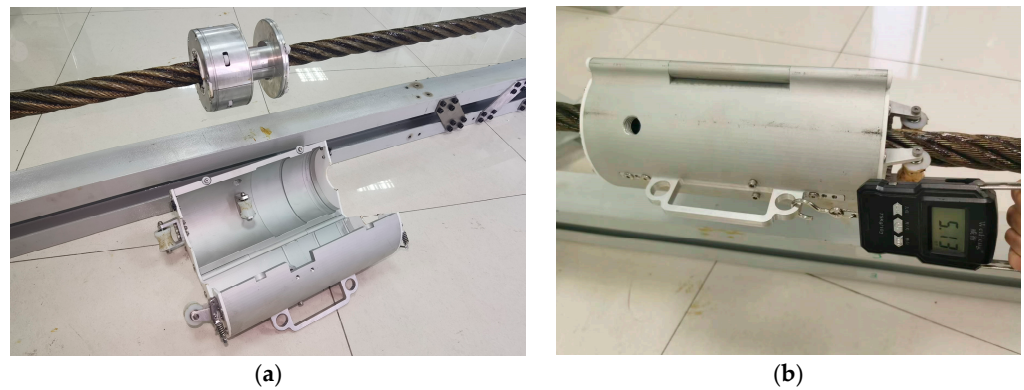
Figure 14. Maintenance device and experimental platform. (a) Before installing the housing module, and (b) the traction test of the wire rope maintenance device.
