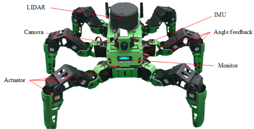
Figure 2. Structure of the hexapod robot.
