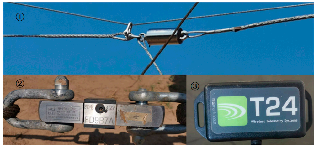
Figure 10. Some experiment devices (①release device,②tension sensor,③wireless communication module).
