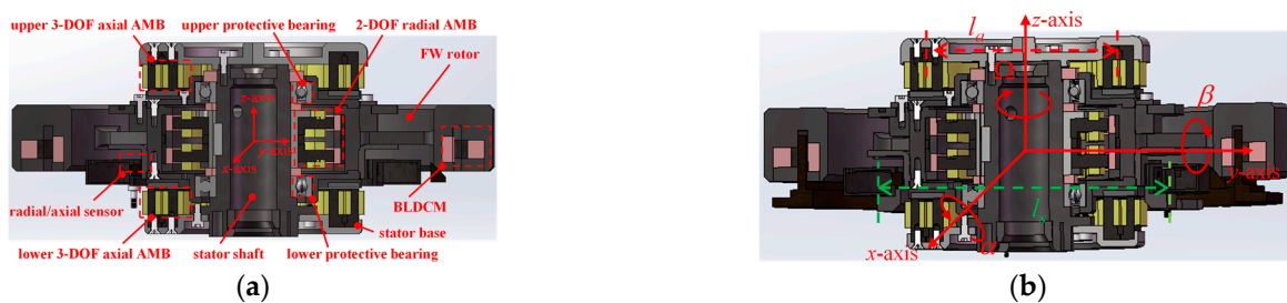
Figure 1. The system view of the 5-DoF MSFW. (a) The main components of the 5-DoF MSMW; (b) the displacement terms of the 5-DoF MSMW.
