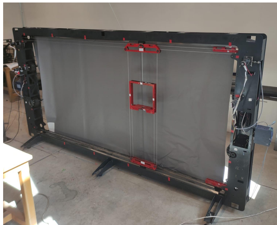
Figure 8. Design and Prototype of the proposed sCDPR.
