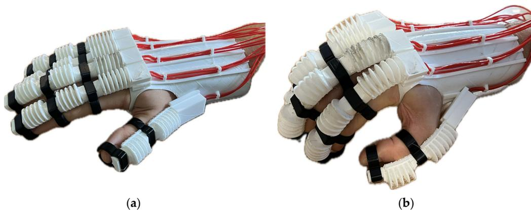
**Figure 5.** Soft-robotic glove fitted to the user's hand: (a) all soft actuators in initial position and (b) all soft actuators activated.
