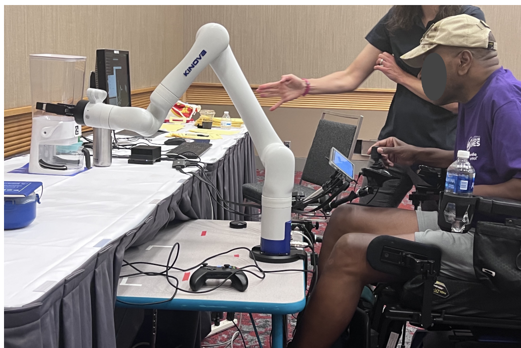
Figure 1. The study setup with robotic arm mounted on table in front of power wheelchair Veteran.
