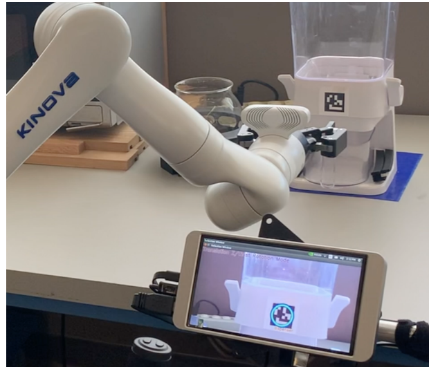
Figure 3. User-Initiated Software Autonomy: The dispenser tag is highlighted on the touchscreen, allowing the user to press a circle to transition to software autonomy.
