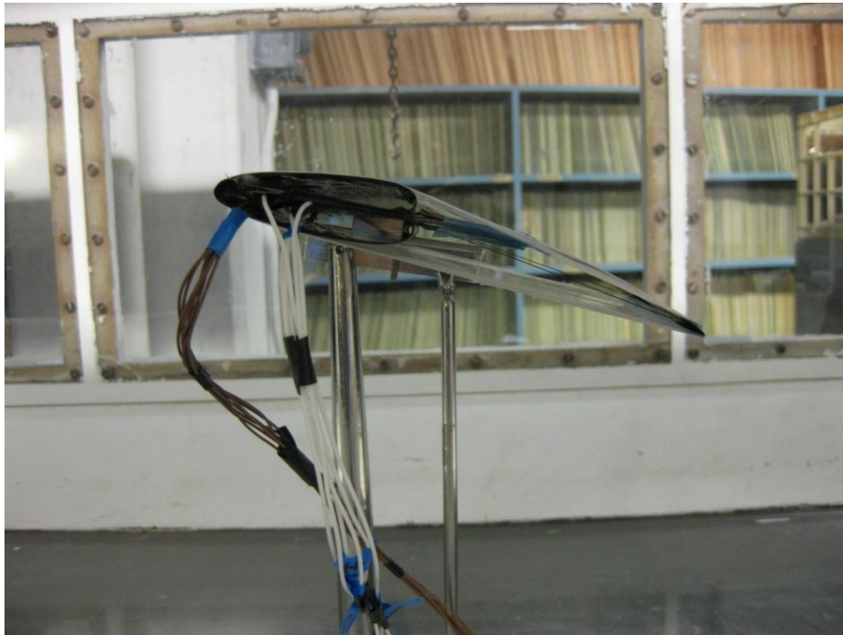
Figure 10. Side view of Airfoil in Wind Tunnel with a Tip Rotation of \delta = 30^\circ .
