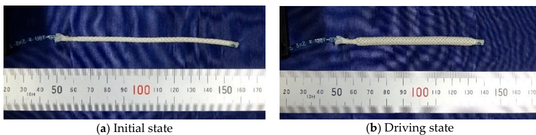
Figure 2. (a) Initial and (b) driving states of the thin artificial muscle.
