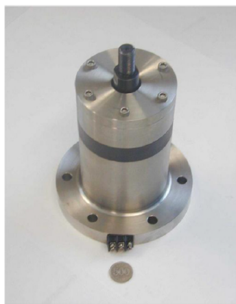
Figure 2. Linear magnetostrictive actuator prototype developed in [75]. Reprinted with permission from [75].
