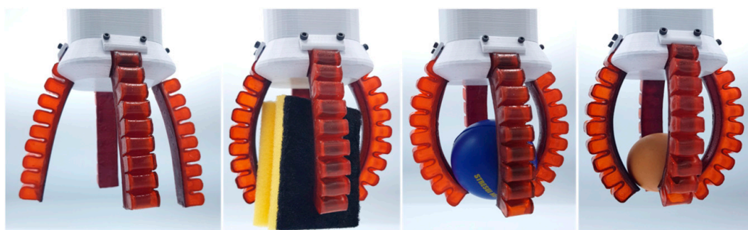
Figure 13. Four BSPAs can work together in a soft gripper that allows picking and placing different objects through pressurizing and depressurizing the air chambers.
