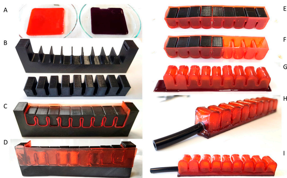
Figure 9. Manufacturing process of the multi-material self-healing bending soft pneumatic actuator constructed out of DPBM-FT5000- r_{4/6} (red) and r_1 (purple).
