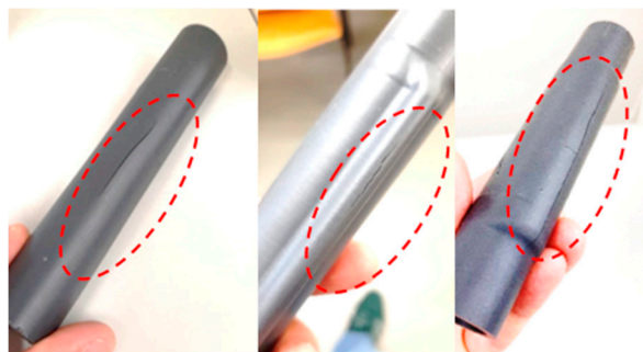
Figure 16. Failure regions in different designs. From left to right: design C, design A and design B.
