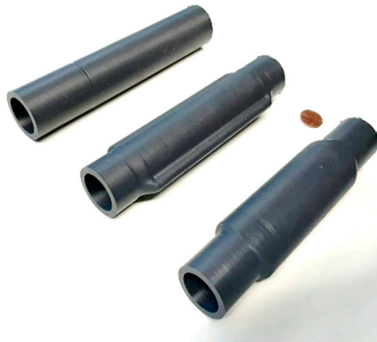
Figure 14. Different 3D printed hose geometries studied in this work. From left to right: Design C, design A and design B.
