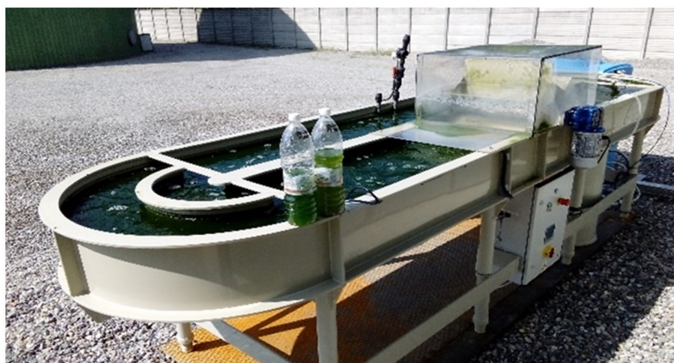
Figure 1. Pilot-scale HRABP located in a piggery farm in the north of Italy (Casaletto di Sopra, Cremona, Italy).
