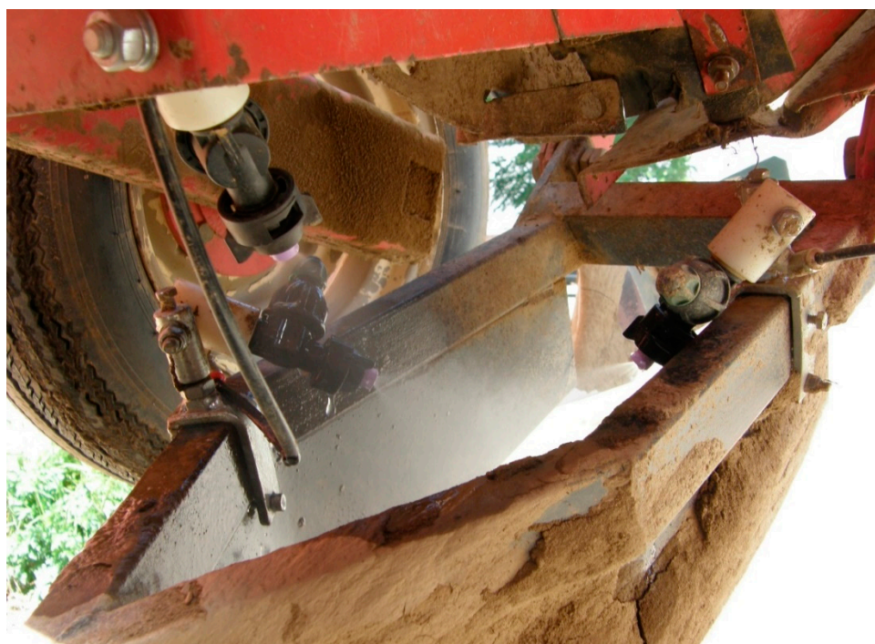
Figure 6. Detail of phage suspension spray application nozzles in the planting machine.
