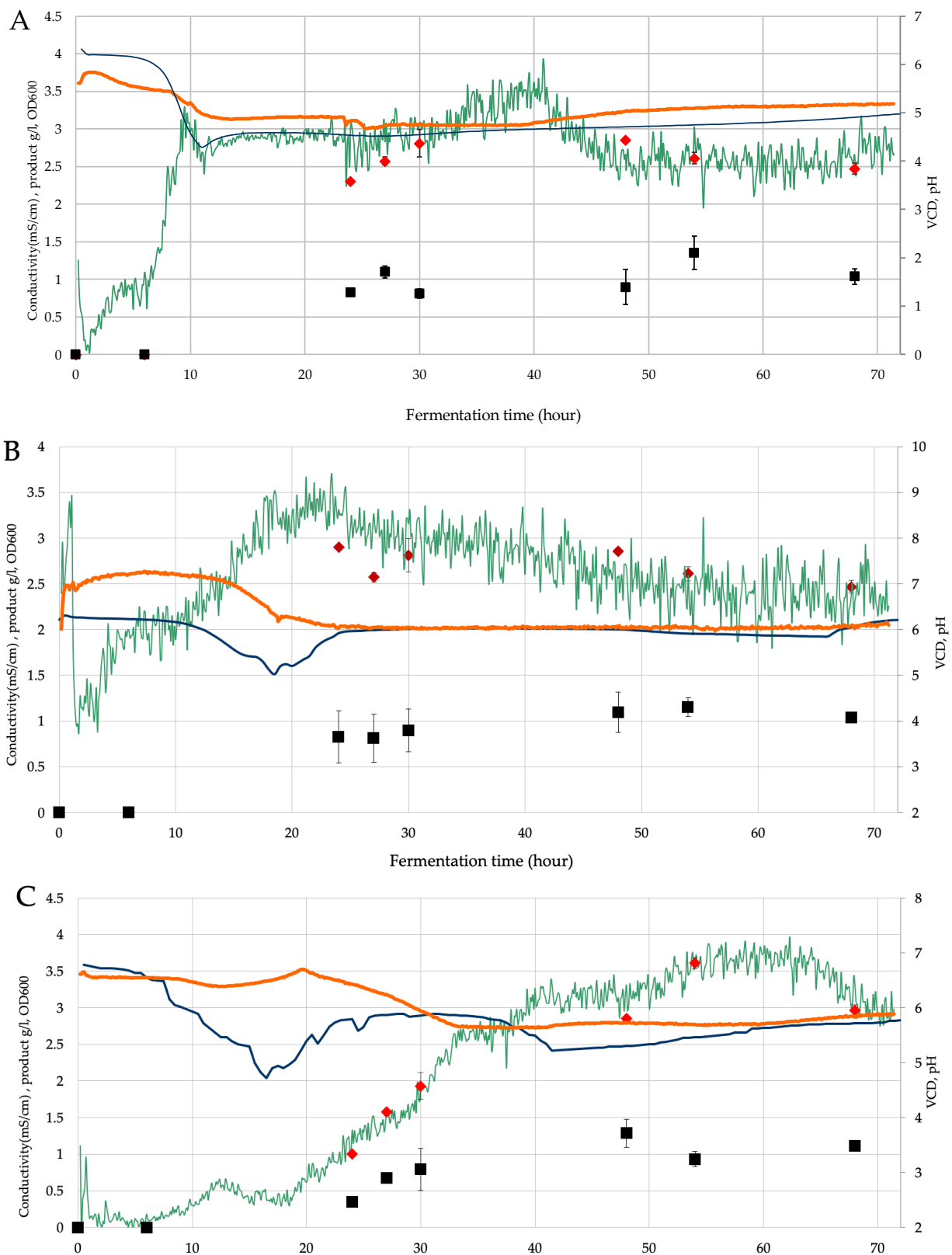
Figure 1. Time course of biosurfactant fermentations: (A) B. licheniformis — In-line detected total products IDTP ( =0.65 \times \text{conductivity [mS/cm]} + 0.1 ); (B) B. subtilis — IDTP ( =0.65 \times \text{conductivity [mS/cm]} + 0.1 ); (C) G. stearothermophilus — IDTP ( =0.65 \times \text{conductivity [mS/cm]} + 0.1 ) biosurfactant fermentation, — pH, — VCD ( =10 \times \text{permittivity [mS/cm]} + 1.8 ), \diamond OD600 and \blacksquare product.
