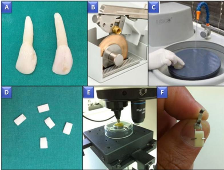
**Figure S1. Enamel and dentin slab preparation.** A. Selected bovine incisors. B. Diamond saw used to cut bovine incisors. C. Polishing a slab in the automatic polisher. D. Dimensioned bovine enamel slabs. E. Measurement of the initial Knoop surface microhardness with the microindenter. F. Mounting an enamel slab in the holder device, secured with composite resin.
