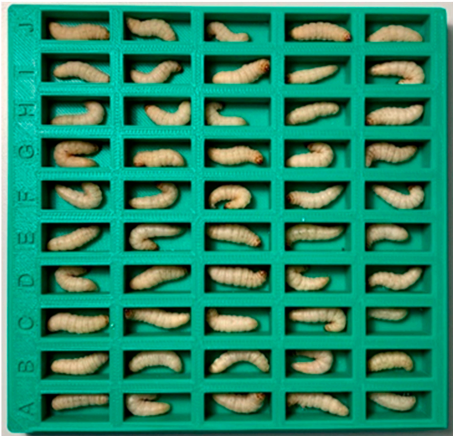
Figure S1. 3D printed plastic trays with wells to separate and contain individual G. mellonella larvae. Plastic lids were securely fitted to the tray to prevent escape during the assay.
