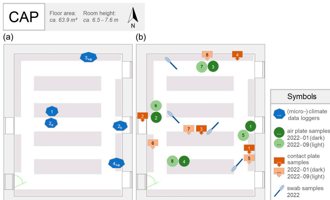
Figure A4. Overview of the library room at Capuchin Monastery (CAP): room measurements, orientation, locations of climate sensors (a) and biological sampling points (b). A more detailed description of symbols is given in the box in the lower right corner.
