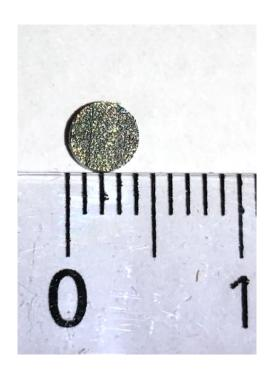
**Supplemental Figure 1**. A sandblasted titanium alloy (Ti6Al4V) disk (diameter 4mm, height 2mm) is depicted
