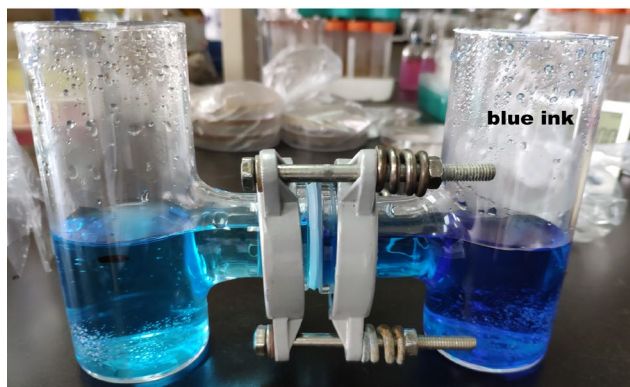
Figure S1 The device for non-contact co-culture. Diffusion of blue ink through a 0.22- \mu\text{m} polyether sulfone membrane from the right compartment to the left was observed within 2 hours.
