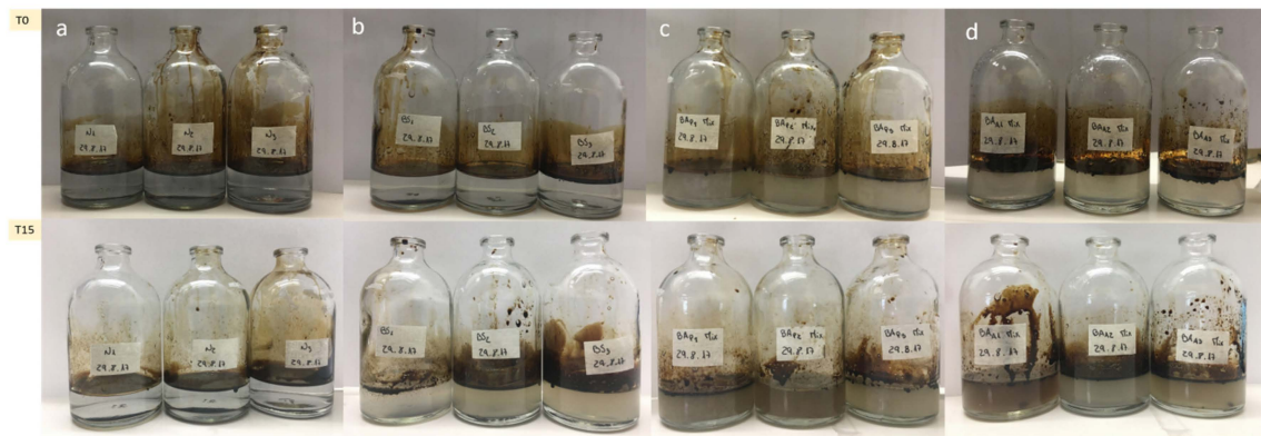
Figure 4. Visual inspection of oil degradation in the beginning (T0) and end (T15) of the bioremediation experiments in controlled laboratory conditions. The four treatments are natural attenuation (a), biostimulation (b), bioaugmentation with inoculum pre-grown in petroleum (c) and bioaugmentation with inoculum pre-grown in acetate (d).
