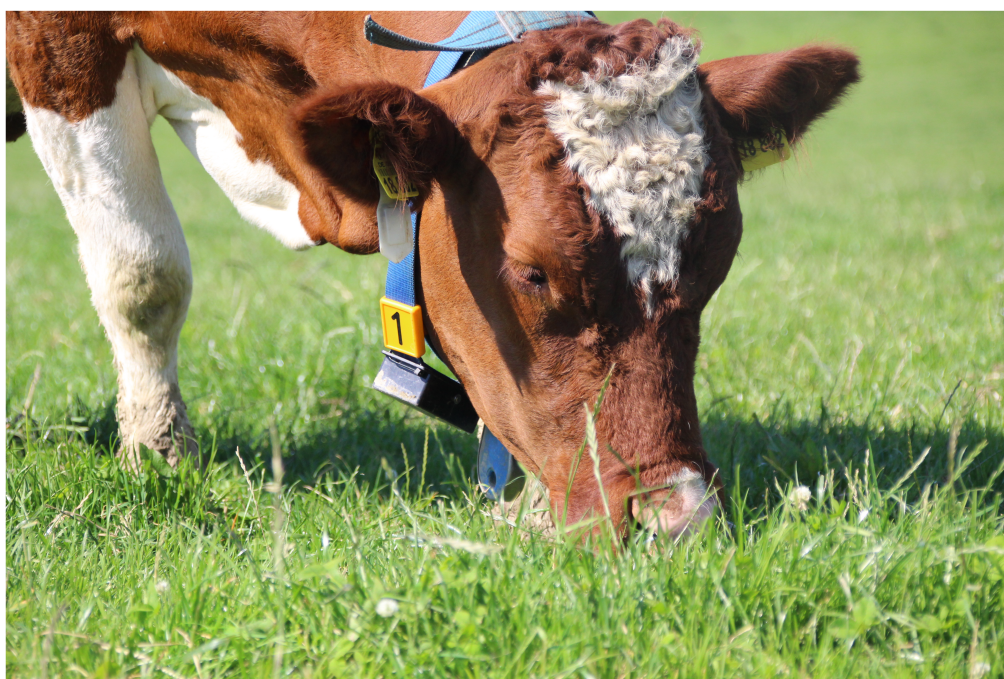
Figure 2. Prototype of the monitoring system (Blaupunkt Telematics GmbH; Hildesheim, Germany) mounted on the collar of a Simmental cow grazing pasture.
