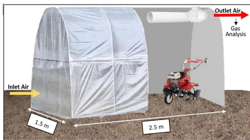
Figure 2. Airtight structure used for dynamic emission. A cut from the inside allows one to see the air extractor as well as the rototiller used to cultivate manure inside the structure.
