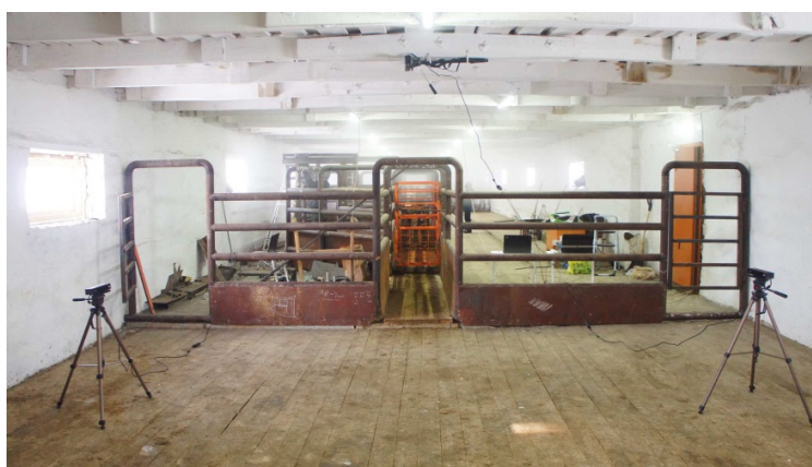
Figure 3. RGB-D image capture system with three Kinect cameras.
