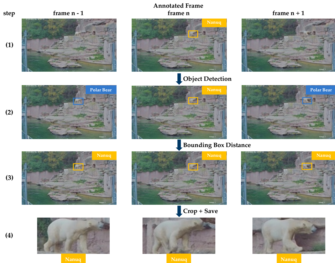
Figure 3. Approach to creating the sequences. For each image labeled by the experts, there is a bounding box including information about the identity of the animal (step 1). The adjacent images are then searched for polar bears in the second step, using an object detection algorithm. To ensure that the correct animal is tracked, we compute the bounding box distances between two consecutive images. If this is below a threshold, we can assign the same ID to the found animal (step 3). In step 4, the bounding boxes are then cropped and saved as a sequence.
