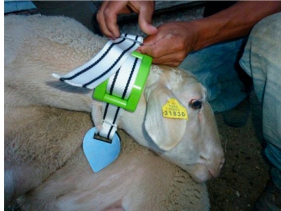
Figure 2. Sheep equipped with GPS device attached to collar.
