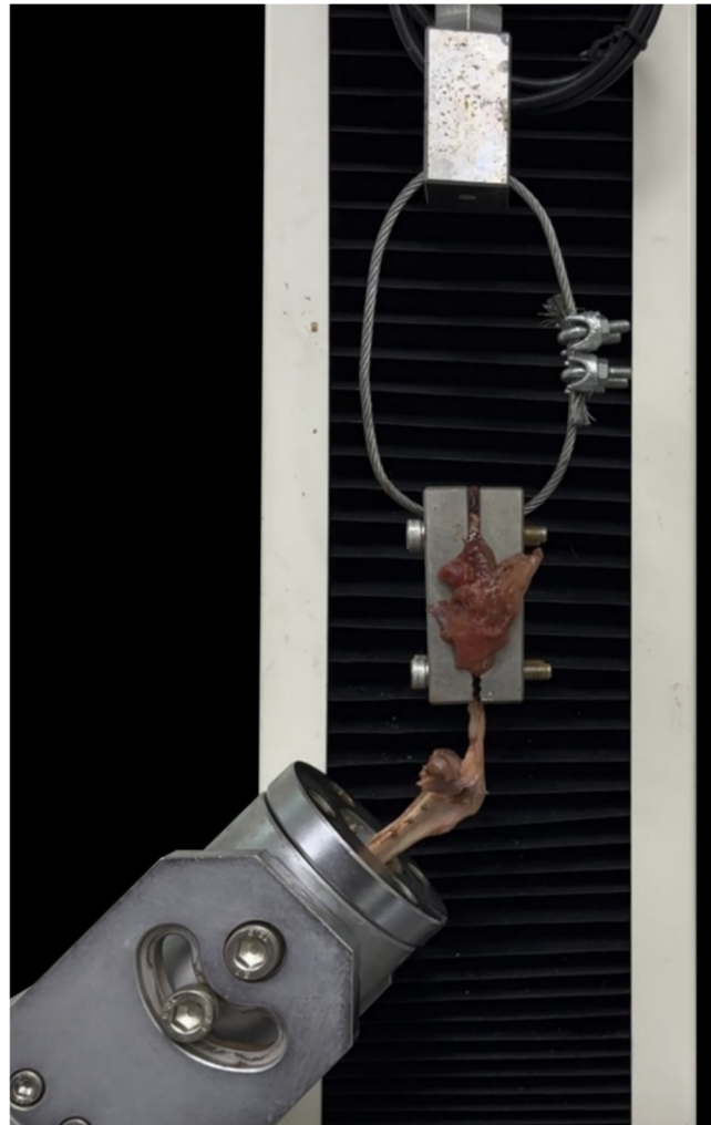
Figure 3. Biomechanical testing setup. Specimens were mounted using methyl methacrylate resin (Trayplast, Vertex, Soesterberg, The Netherlands) in a stainless steel pipe with an inner diameter of 35 mm. The specimens were secured to the loading cell, and the patellar tendon was fixed at an angle of 135° in a custom-designed clamp.
