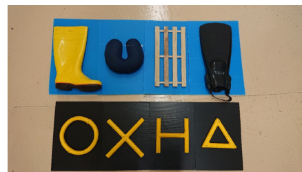
Figure 4. Four “realistic patterns” attached onto blue plastic cardboards and four “geometric patterns” attached onto black plastic cardboards.
