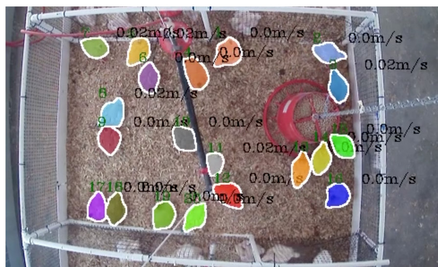
Figure 5. Track and detection speed of broilers (the green number indicates the tracking number, while the black number represents speed).
