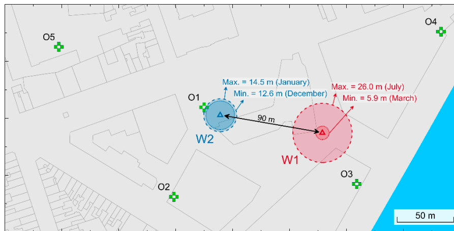
Figure 8. Maximum and minimum thermal radii of the ATES well doublet (W1–W2).
