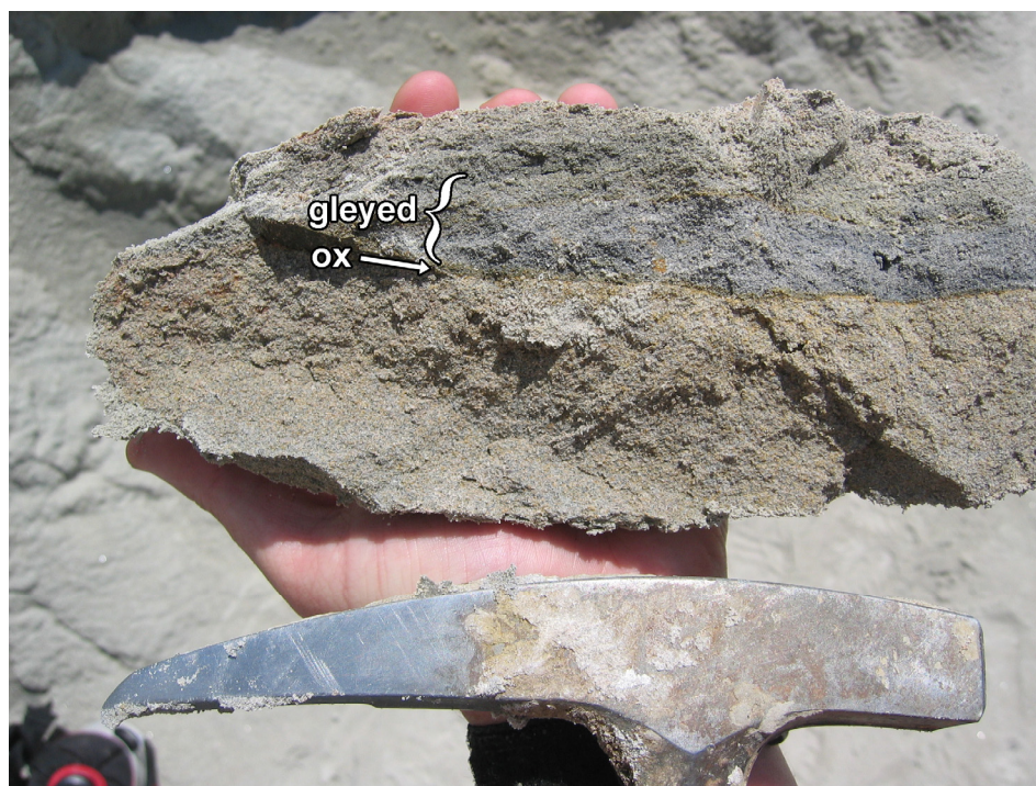
Figure 9. Close-up photograph of the contact between the upper pale unit, and lower tan unit of the Colgate Sandstone. Note the thin (1 mm) iron-rich oxidation zone (ox) at the contact, and overlying 2 cm grey gleyed zone (gleyed) in the upper unit. Hammer head length: 17 cm. Photo taken at Crooked Creek, near Winnett, Garfield Co. MT, 47°24'13'' N, 108°14'35'' W; (NAD27CONUS).
