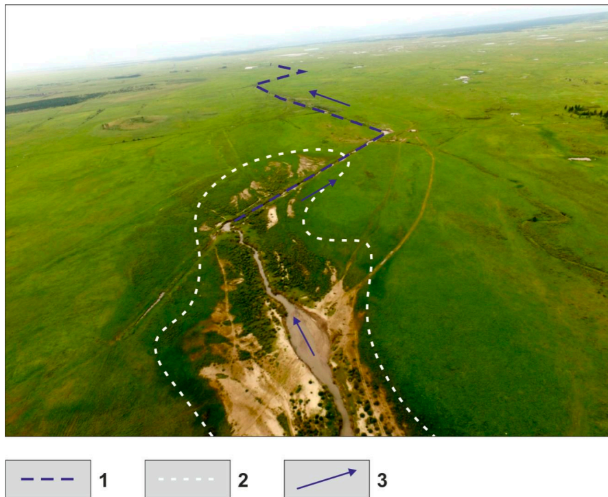
Figure 13. Zone of accumulation of suspended load on the Kyngarga river where it enters the dike. Images were taken on 12 July 2017, from the Phantom 3 quadcopter, at 234 m (51°51′5.36″ N, 102°27′20.09″ E). 1: boundary of accumulation of suspended load; 2: dike; 3: direction of the river.
