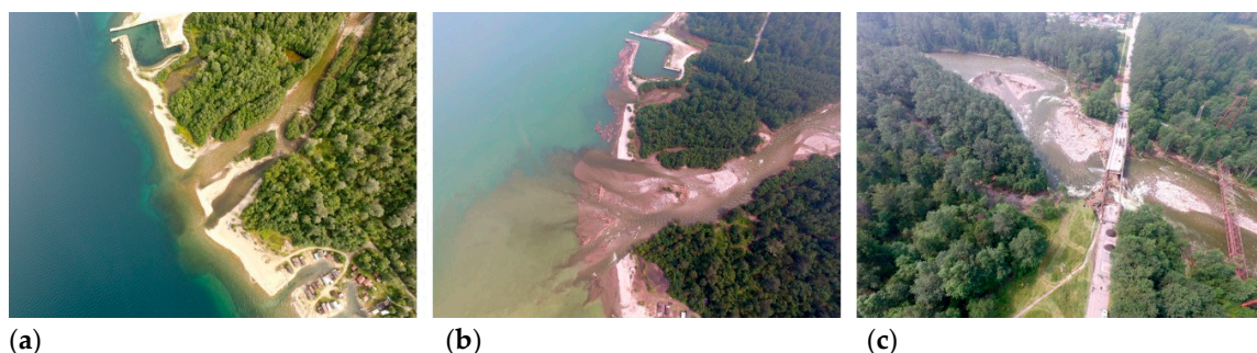
Figure 16. The consequences of the flood on the Solzan river. (a), (b) channel morphodynamics at the mouth of the river. Coordinates: 51^{\circ}31'46.6418'' N, 104^{\circ}9'27.5627'' E. Images was taken: (a) 23 August 2017, (b) 31 July 2019; (c) the destroyed technological bridge. Coordinates: 51^{\circ}31'24.6506'' N, 104^{\circ}9'43.3299'' E. Images was taken on 31 July 2019.
