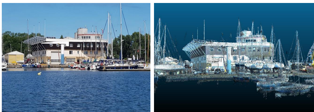
Figure 12. The image seen by the navigator and its construction on the basis of geospatial data from TLS cloud.
