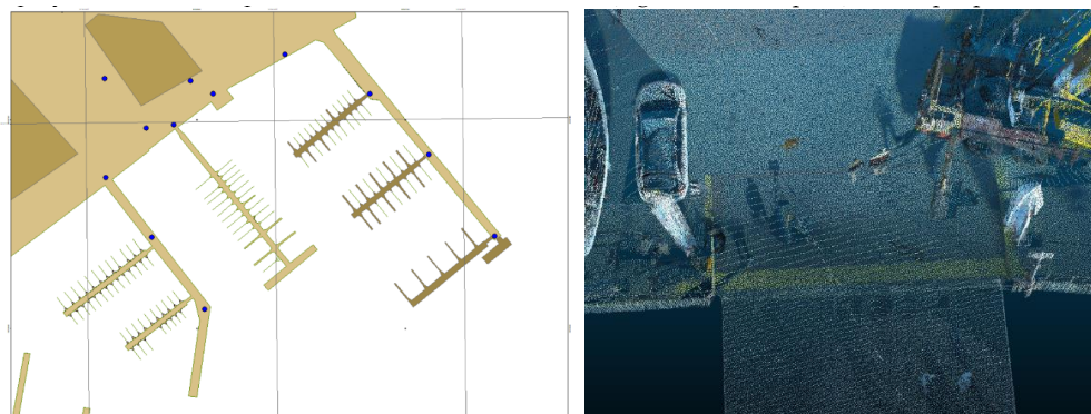
Figure 7. A part of TLS stations (left) and visualization of one of them close to slipway (right).
