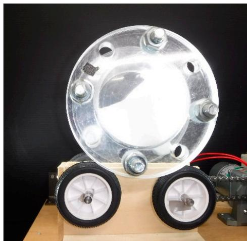
**Figure 1.** Rotating drum used in this study. An acrylic cylindrical container is set on a turntable.
