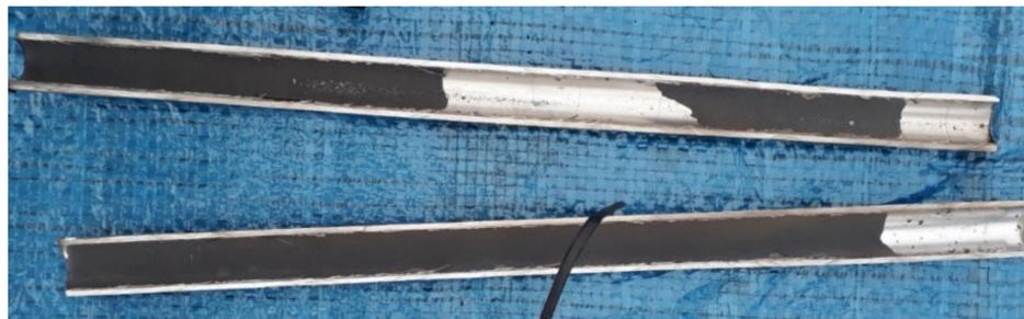
**Figure 3.**  $\text{PbS}$  scales deposited in tubes from the test heat exchanger.
