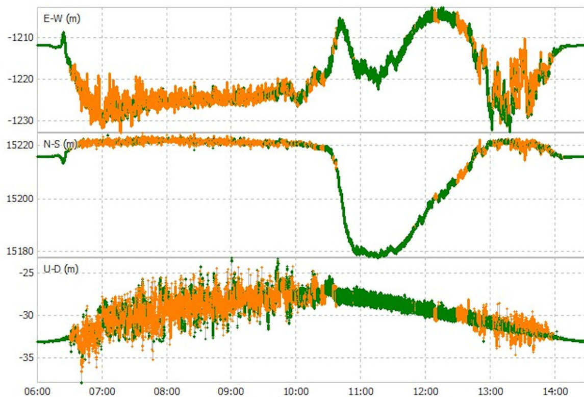
Figure 6. Buoy positional components during tidal cycle B; East–West (E–W), North–South (N–S) and Up–Down (U–D), August 29 2019 06:00–14:00. Fixed solutions (Q1) are shown in green, and float solutions (Q2) are shown in orange.
