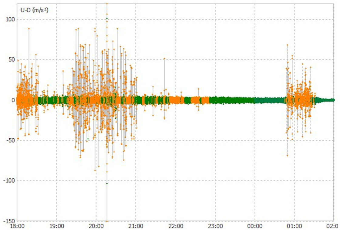
Figure 7. Buoy vertical accelerations during tidal cycle A; 18:00 28 August–02:00 29 August. Fixed solutions (Q1) are shown in green, and float solutions (Q2) are shown in orange.
