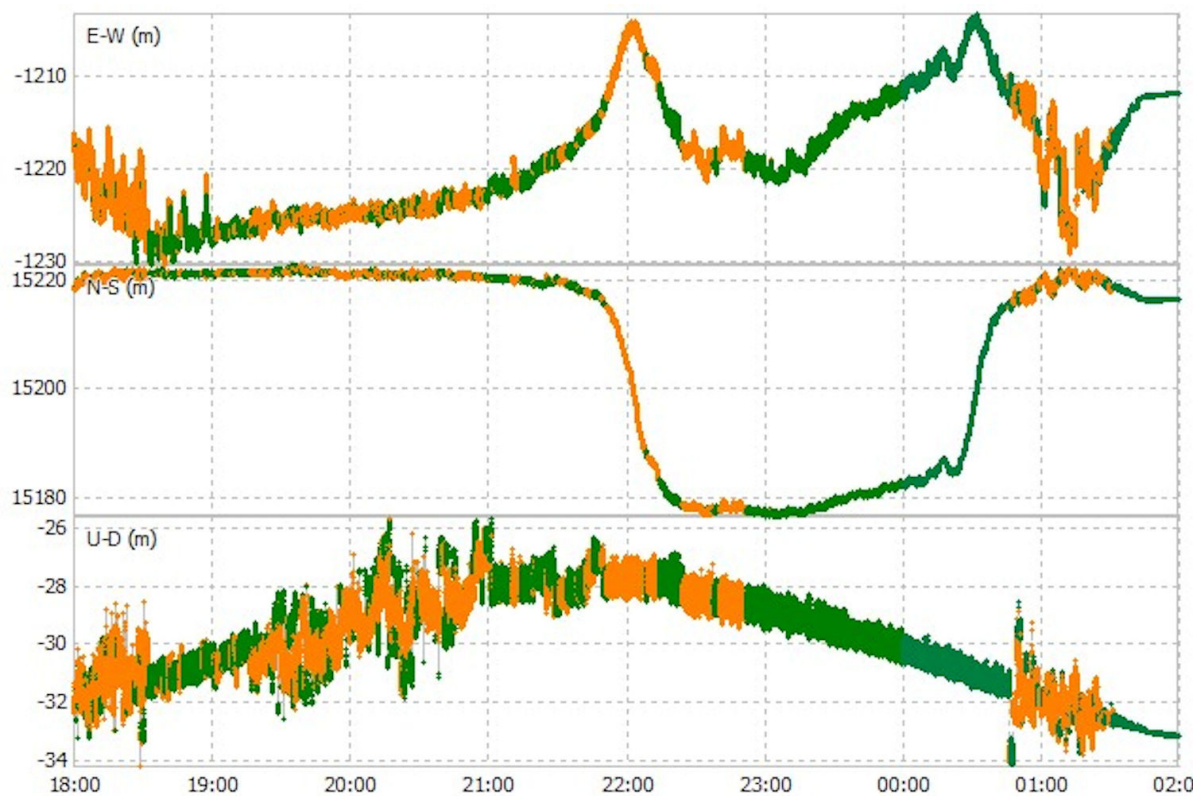
Figure 5. Buoy positional components during tidal cycle A; East–West (E–W), North–South (N–S) and Up–Down (U–D), 18:00 28 August–02:00 29 August. Fixed solutions (Q1) are shown in green, and float solutions (Q2) are shown in orange.
