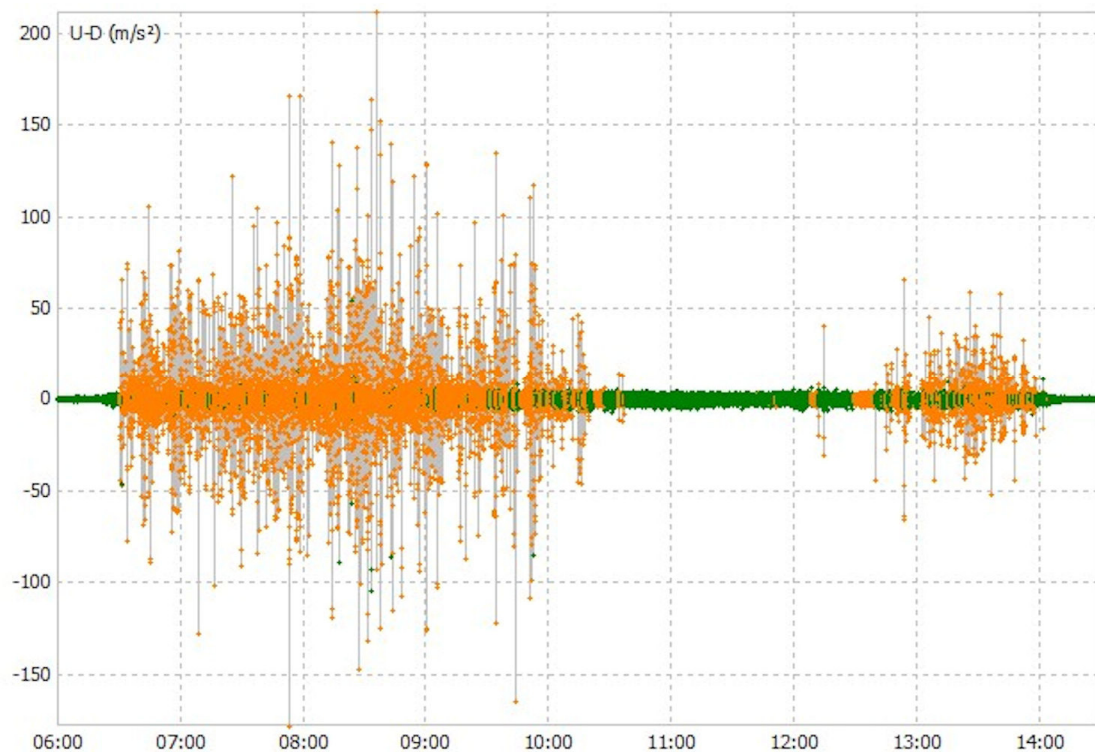
Figure 8. Buoy vertical accelerations during tidal cycle B; Up–Down (U-D), 29 August 06:00–14:30. Fixed solutions (Q1) are shown in green, and float solutions (Q2) are shown in orange.
