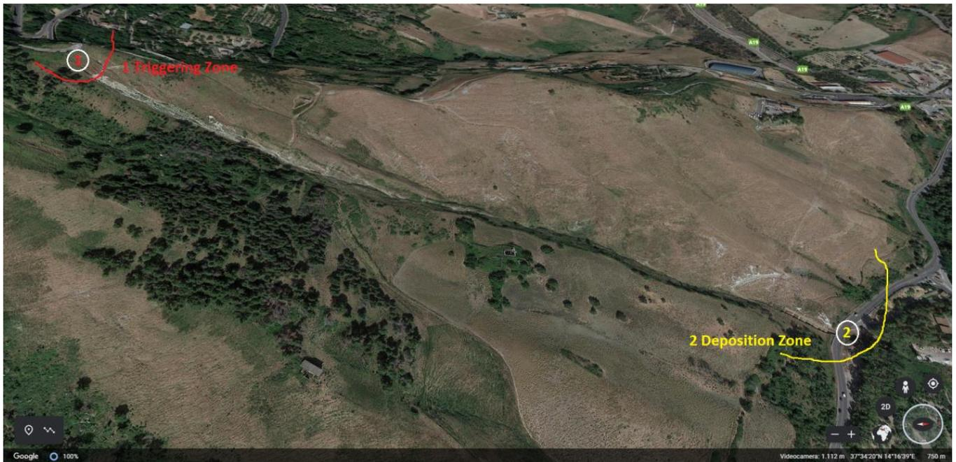
**Figure 17.** Location of the triggering (1) and deposition (2) zone of the debris flow.
