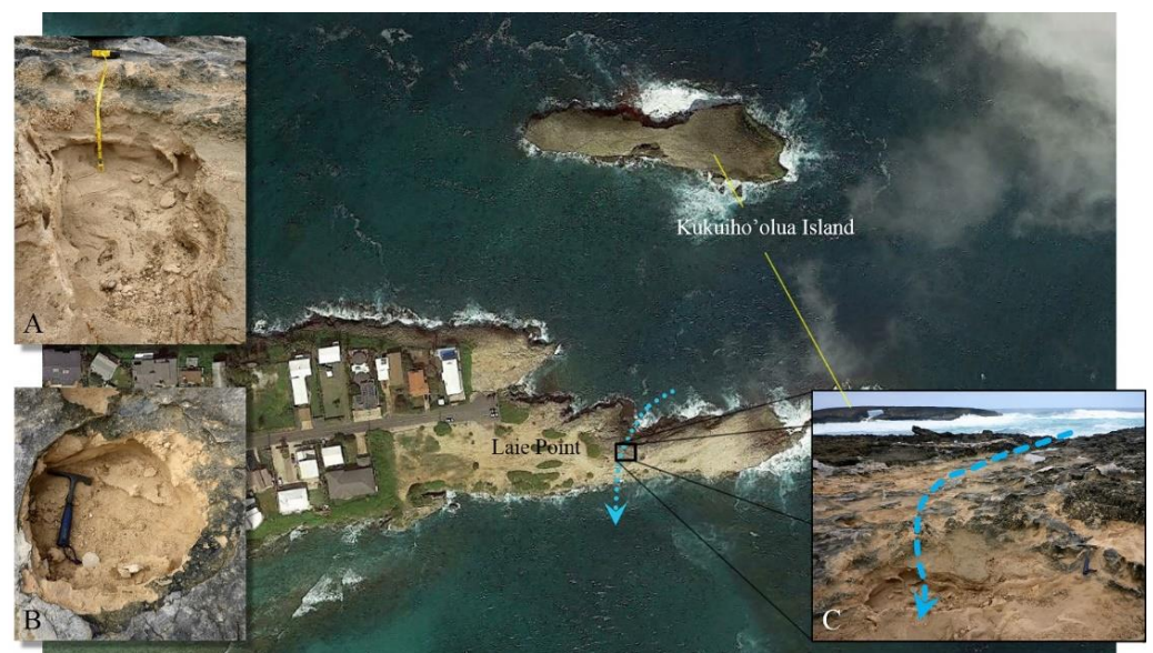
Figure 5. Evidence for waves over-topping the peninsula at Laie Point, Oahu. Examples include oxidized surface removal (C) and erosion pits (A,B). View in C is looking north. Arrow indicates likely flow path of seawater. Base map from Google Earth.
