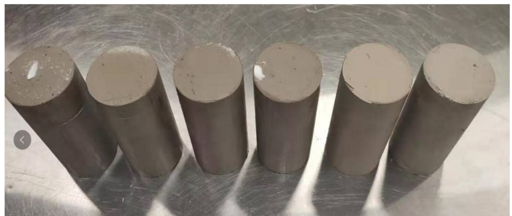
Figure 3. Examples of some cement-stabilised specimens for unconfined compressive strength tests, Port of Brisbane Soft Soil + 5, 10, 15, 20, 25, and 30% cement, respectively.
