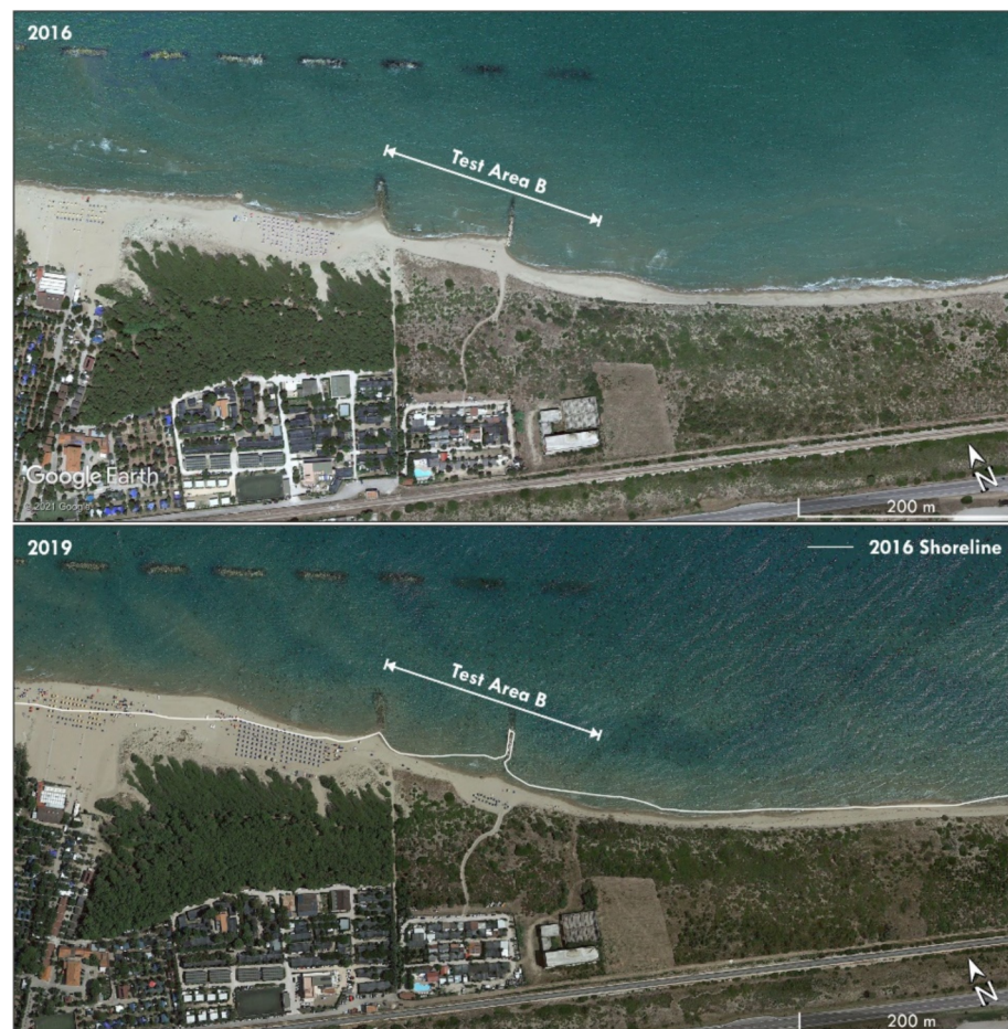
Figure 8. Evidence of shoreline and beach changes from 2016 to 2019 (Google Earth images dating back to 20 June 2016 and 20 July 2019) along the coastal stretch that includes test area B. On the Google Earth image from 2019, the white line indicates the shoreline of 2016.
