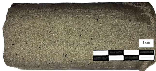
Figure 2. General view of the frozen sand 3 sample with pore methane hydrate ( W = 14\% ; S_h = 26\% ; T = -6\text{ }^\circ\text{C} ).
