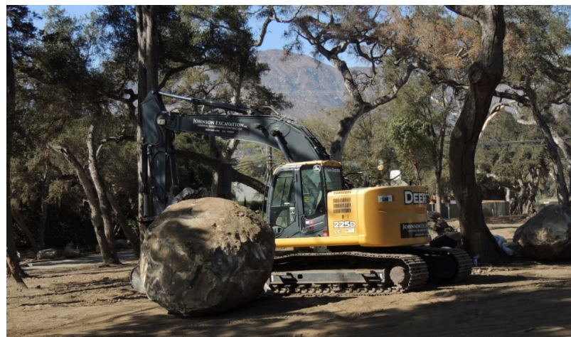
Figure 8. Boulder transported by Montecito debris flow that is larger than the local channel dimensions (max clast size/channel width > 1).
